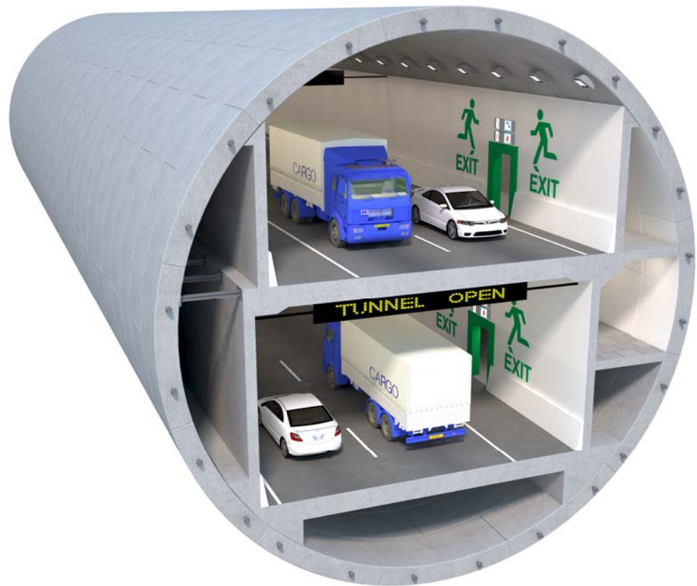
Figure 2. Bored Tunnel Cross-Section
