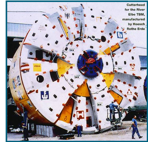
Elbe Tunnel Slurry Machine
