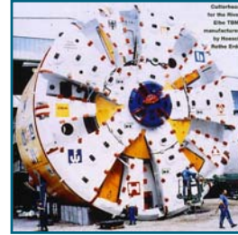
Elbe Tunnel Slurry Machine
