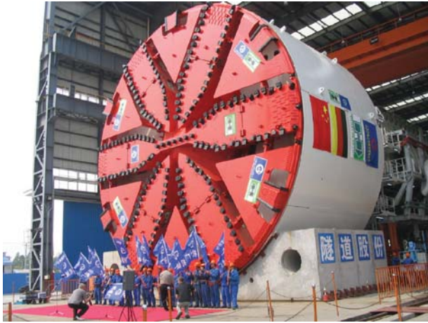
Figure 2. World's largest Mixshield Ø15.4 m for Shanghai.
